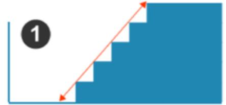
**Measurement 2:** Measure from the edge of the upper landing (like Measurement 1) to the edge of the first stair's tread at the bottom.
